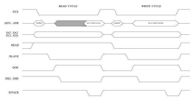
Figure 3-1: Basic Zorro III Cycles
