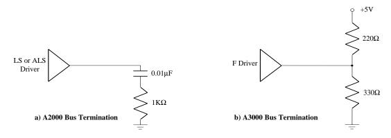
Figure 2-1: A2000 vs. A3000 Bus Termination
