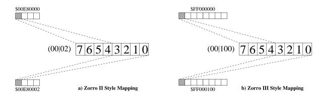
Figure 8-1: Configuration Register Mapping
