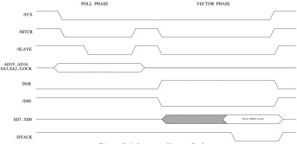
Figure 3-4: Interrupt Vector Cycle
